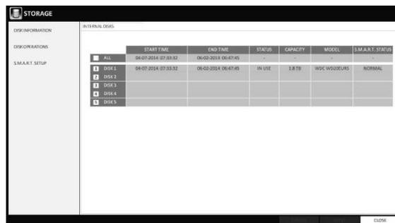
The screenshot shows the 'STORAGE' menu with 'INTERNAL DISK' selected. A table displays SMART information for five disks. Disk 1 is 'IN USE' and has a 'NORMAL' SMART status. Disks 2, 3, 4, and 5 are 'NOT IN USE'.
